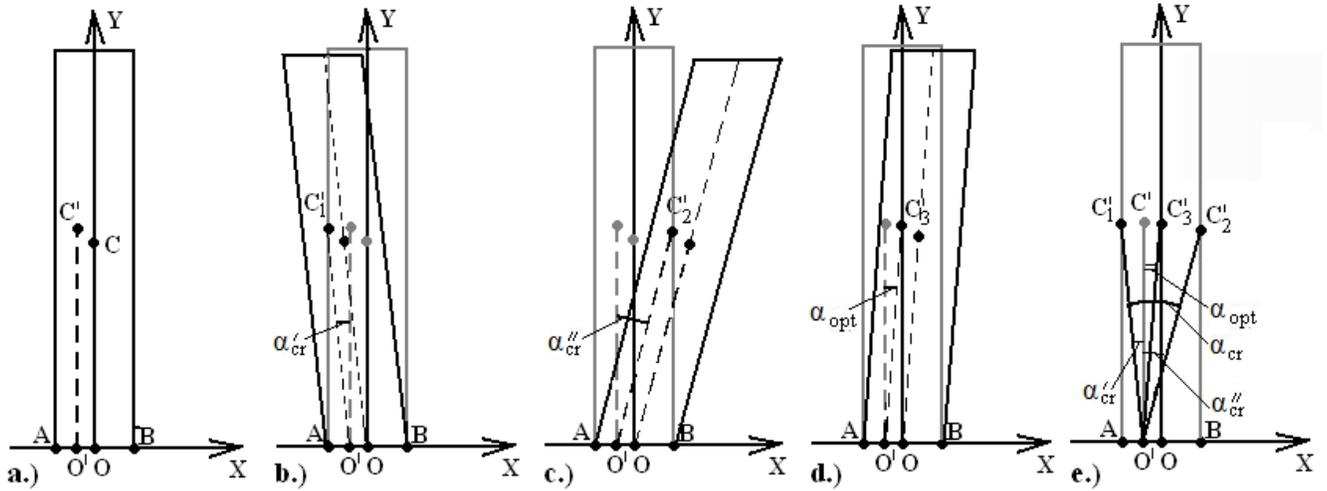
**FIGURE 5.** Different positions of a straight human body: a.) upright position, b.) critical position during backward leaning, c.) critical position during forward leaning, d.) the most stable position of the body, e.) comparative diagram for the positions shown in Figures a.) - d.).
